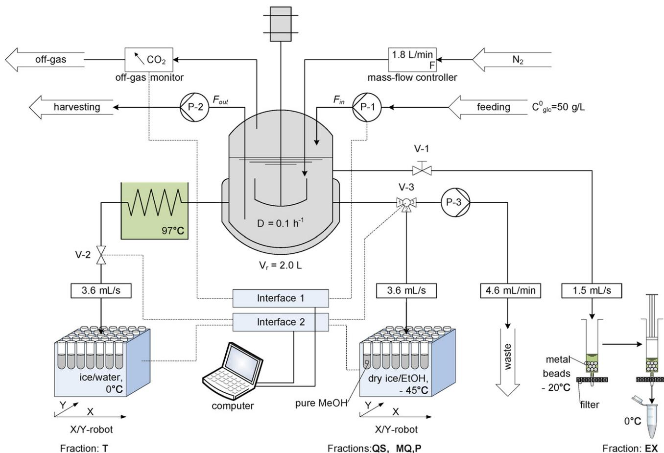
Fig. 1. Scheme of the experimental setup.
